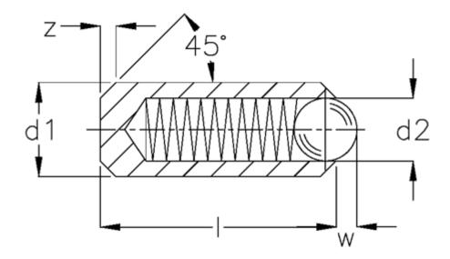
$\begin{array}{ll} d1 & = 5.0 \\ d2 & = 3.5 \\ I & = 13 \\ Spring pressure N bottom = 18.0 \\ Spring pressure N top & = 11.0 \\ W & = 1.00 \\ z & = 0.25 \end{array}$
